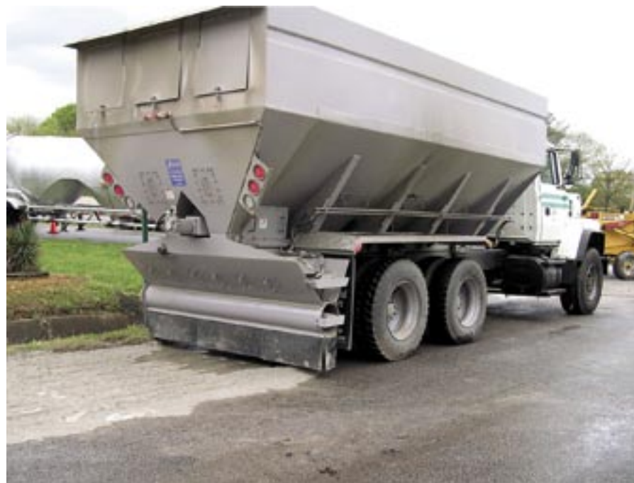
Recupero integrale – posa del cemento sulla vecchia strada tramite spanditrice Full Depth Reclamation - cement spreader truck dropping cement on the old road
